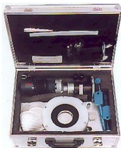
Figure 1 Apparatus for establishing chloride diffusion coefficient
